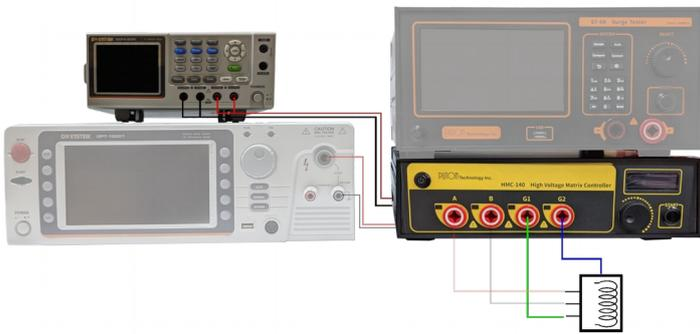
The high-voltage matrix controller is connected to the low-resistance meter for ground continuity test, with PASS/FAIL displayed on the upper right corner screen of the controller.
