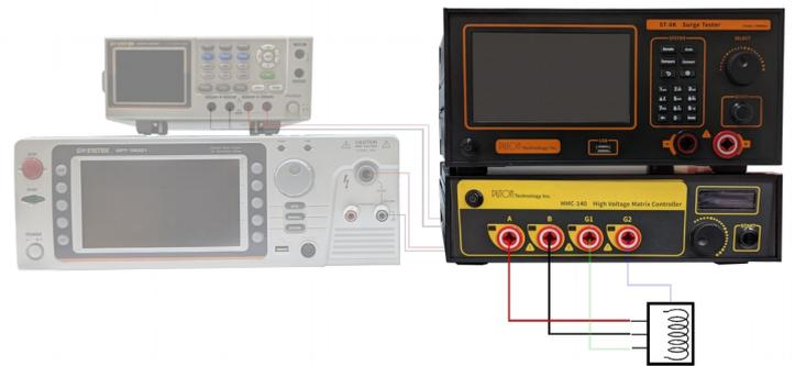
The high-voltage matrix controller is connected to the pulse coil tester for interlayer short-circuit test, with PASS/FAIL displayed on the upper right corner screen of the controller.
