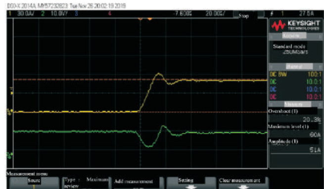
Current rise wave of certain brand electronic load at full speed
